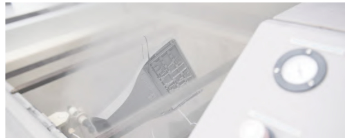
2. Aggressive atmosphere (salt fog - corrosion test)
